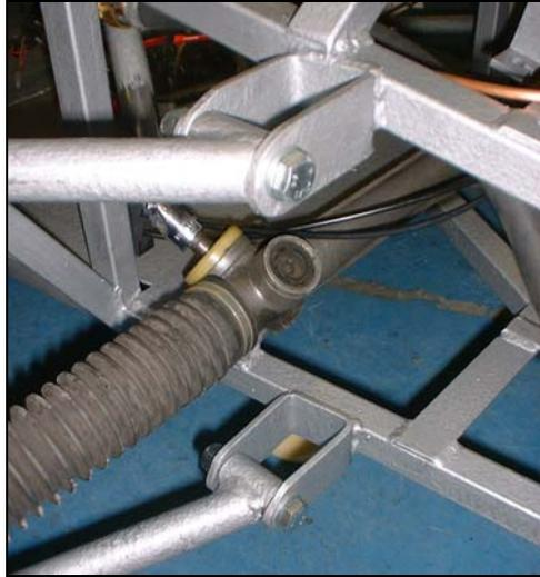
**Figure 1.2 – Wishbone Mounting Brackets**
