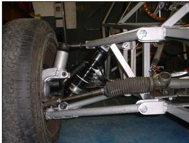
**Figure 1.6 - Front Wishbone Assembly**
