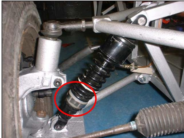
**Figure 1.5 – Suspension Strut Spacer**
