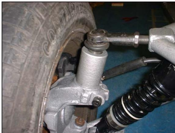
**Figure 1.3 – McPherson Strut & Ball joint**
