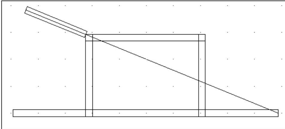
**Figure 1.4 – Ideal Loaded Front Wishbone Position**
